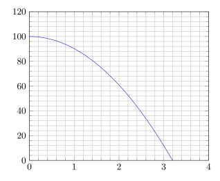
The horizontal axis is in units of seconds (s), and the vertical axis is measured in meters (m). You can interpret the graph as depicting what happens over time when you drop a ball from 100 meters high.
